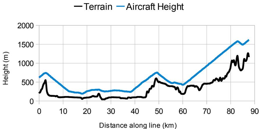
Figure 3: Flight line showing the aircraft "drape flying" to stay close to the terrain while collecting gravity data.
